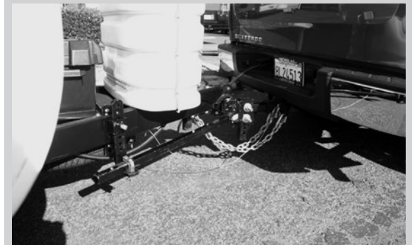
Figure 3 - The A-frame of a conventional travel trailer attached to the rear of a pickup truck.
