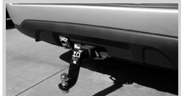
Figure 4 - The draw bar above is a 2-1/4 inch drop. The draw bar below is a 6 inch drop.
