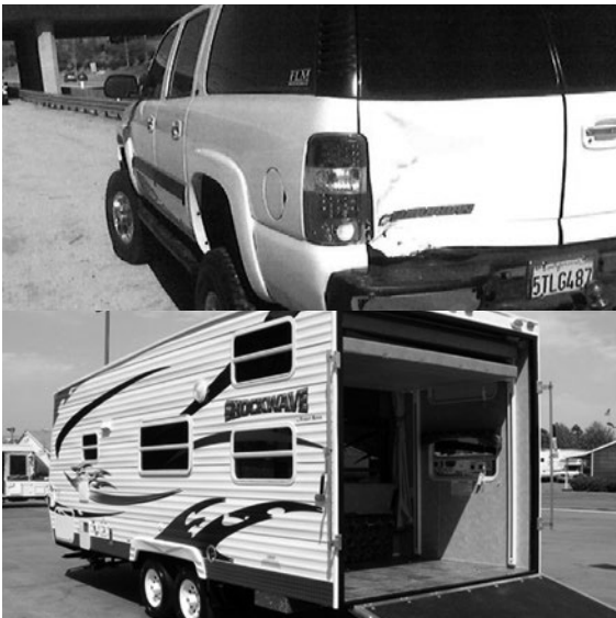
Case Study #2 - The Suburban is shown above. Damage is shown at the rear door and bumper. The trailer shown in the Figure is an exemplar.
