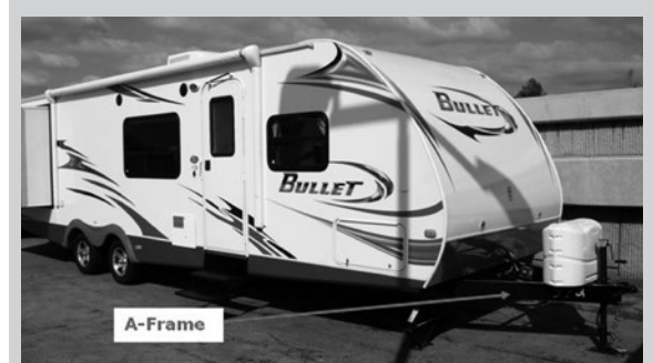
Figure 2 - Conventional travel trailer showing A-frame and A-frame equipment.
