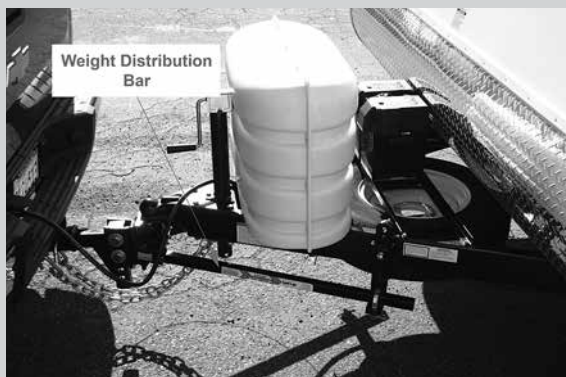
Figure 12 - The weight distribution bar attached to the hitch and the trailer A Frame.
