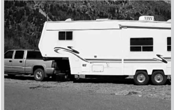
Figure 2 – Fifth wheel trailer shown attached to a pickup. The goose neck at the front of the trailer extends over the pickup's cargo bed. The king pin connects to a hitch mounted in the truck bed.
