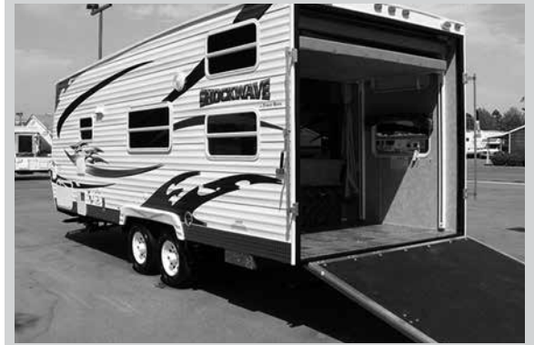
Figure 5 – Sport Utility Trailers have a storage area for transporting vehicles. The rear door folds down into a ramp in order to load the vehicles.
