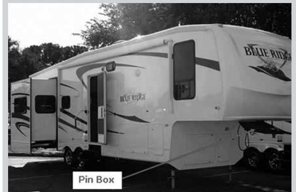
Figure 1 – Fifth wheel showing the gooseneck. The pin box is at the front of the trailer. A king pin is attached to the pin box.
